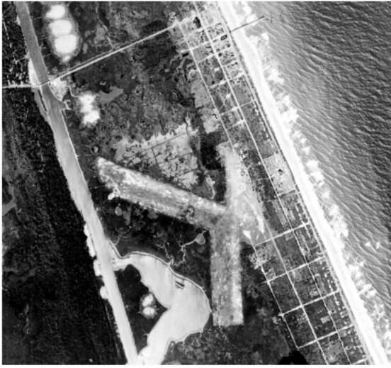
1 A February 12, 1943, U.S. Department of Agriculture (USDA) aerial photograph of the Flagler Beach Airport, much expanded from its original construction in 1929. There were two grass runways. The northwest-to-southeast runway was 3,200 feet long, and the north-to-south runway was 3,000 feet long. That oddly shaped body of water between the Intracoastal Waterway channel and the runways was known as Stomach Lake. (Credit: The University of Florida Map & Imagery Library)
