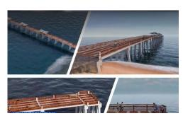
Construction of the new proposed pier is expected to begin in the summer of 2024 and will take a few years to complete. As proposed, the new pier will be 828 feet long, its historic length. The first 82.5 feet of the existing wooden pier will be repaired and retained connecting to the new construction that is 715 feet long by 25 feet wide. The new pier will have a 20-foot-long T-head which would be 32 feet wide. The new pier will be 28 feet above the water while the existing pier is
